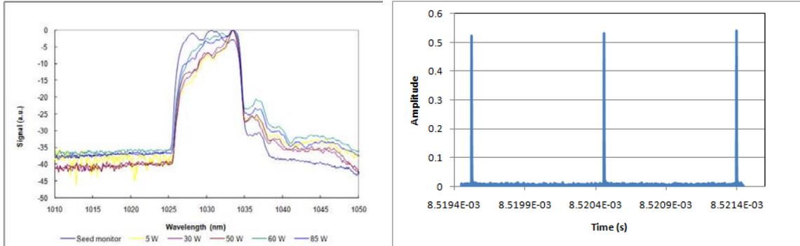
Figure 3 Spectra and pulse train of MHz high power/energy fs fiber laser
