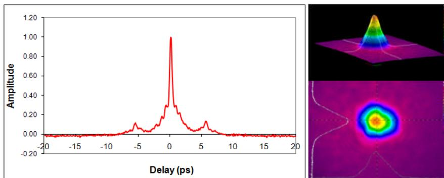
Figure 4 Pulse train and beam profile for 100 W and 100 micro-J operation. The satellite pulse comes with the nonperfect PM PCF fiber design (PM: polarization maintaining).
