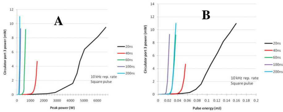
Figure 1 SBS Power (from Circulator Port 3) as a functions of: A) Output peak power; B) Output pulse energy.
