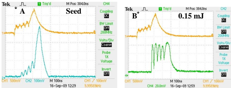
Figure 2 Manipulating seed pulse shape to generate ~200 ns amplified pulses. A) Seed shape; B) At 0.15 mJ (8.6 A), ~200 ns macro-pulse width with flat top was obtained.
