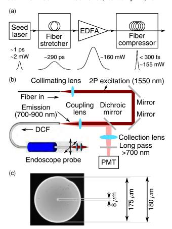
Fig. 1. (Color online) System design and components: (a) block diagram of the  $1.55\,\mu\mathrm{m}$  short-pulsed fiber laser, (b) detailed layout of the optical path, (c) micrograph of the double-clad fiber cross section.
