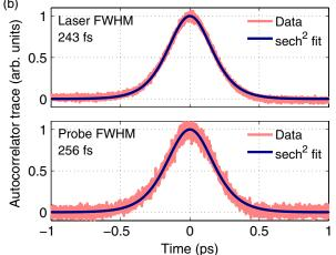
Fig. 2. (Color online) (a) Spectra and (b) autocorrelation traces of the pulses at the laser output and at the endomicroscope output.
